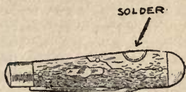
A PIECE OF SOLDER FASTENED TO THE METAL OF THE KNIFE HOLDS THE BROKEN-OFF HORN IN PLACE.
